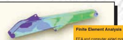
FEA and computer aided motion analysis allows the boom to be signed, tested, simulated and improved before the manufacturprocess begins. Associative software ensures superior partwhich means stronger, trouble-free equipment
